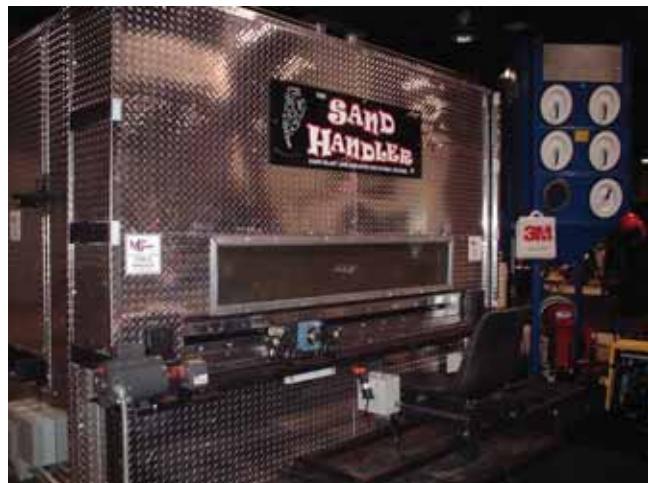
Miles Supply Co. brought its latest manual sandblast machine which includes the abrasive recovery system. This is the only sandblast machine on the market where the operator actually can move with the curtain and be in the comfort of a seat. The room can blast 7 feet horizontal and 4 feet vertical, and retails for $19,500.
