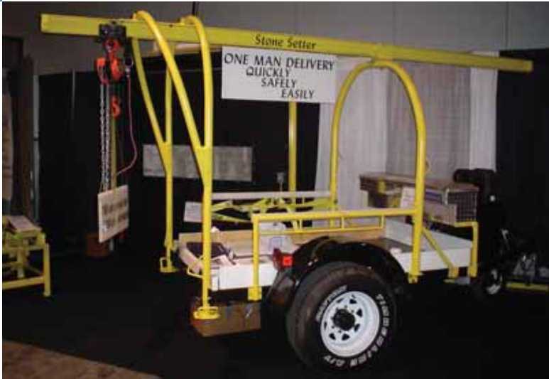
Hiron's introduced its Stone Setter, a powered trailer designed to lift and carry monuments.
